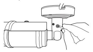
To open the camera from panel to have access to the lens focus 4 and zoom and also to the local storage slot please remove the sun hood and by pressing the camera body down against a solid surface rotate the lock ring clockwise.
