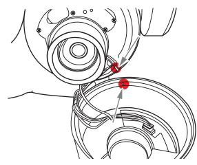
Once the housing front ring has been aligned close the ring Once the camera is correctly installed follow the camera user 8 manual to have access to the setting interface.
