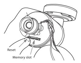
6 To close the camera front part please align correctly the flanges with the grooves; avoid cables to be damages while closing the camera.
