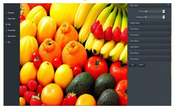
OSD function enable user to add, modify and delete image's all text including device time. User can adjust image's front size and front transparency at [Basic Setup] pull-down menu. User can add device name, adjust time display sequence and control at [System Setup] item.
