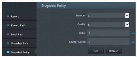
Select **[Number]** pull-down menu, adjust snapshot quantity as trigger snapshot each time and user can snapshot 1-6pcs image for each time snapshot.
