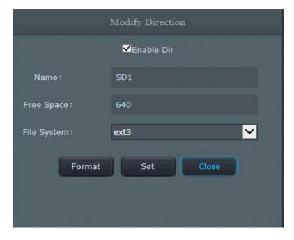
Select **[Enable Dir]** to start SD card recording function.
