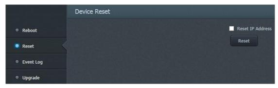
User can click reset button to reset system configuration parameter in this interface and also can select **[Reset IP]** to reset device to default.
