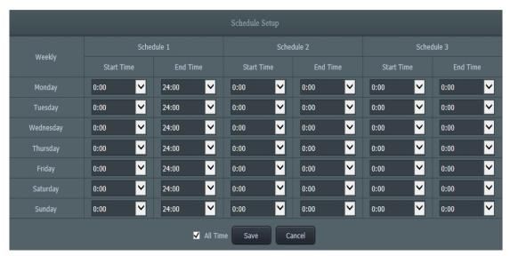
Select **[All time]** to set up motion detection as all-time detection. And also select time at schedule to complete time setup. At last click **[Save]** to finish time setup.
