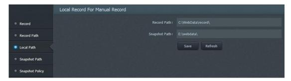
User can set up local recording path and snapshot storage path by disk path. Click **[Save]** to save settings.
